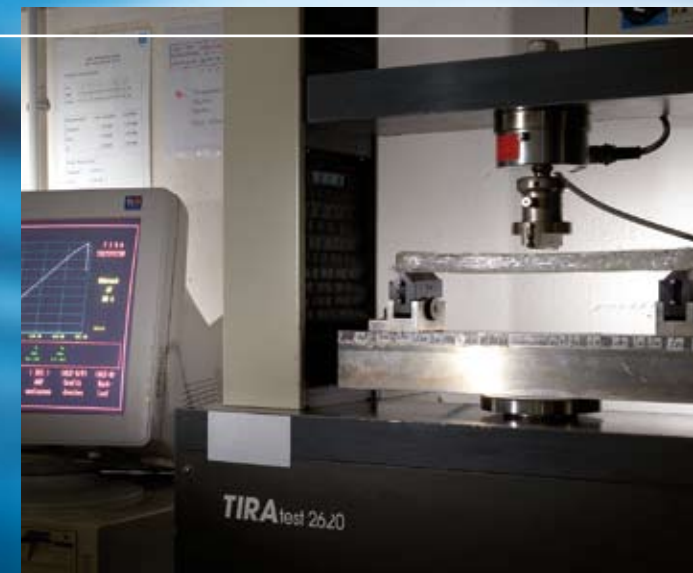
Loading test: Sight glasses from every toughening batch are tested in the very latest testing apparatus.
