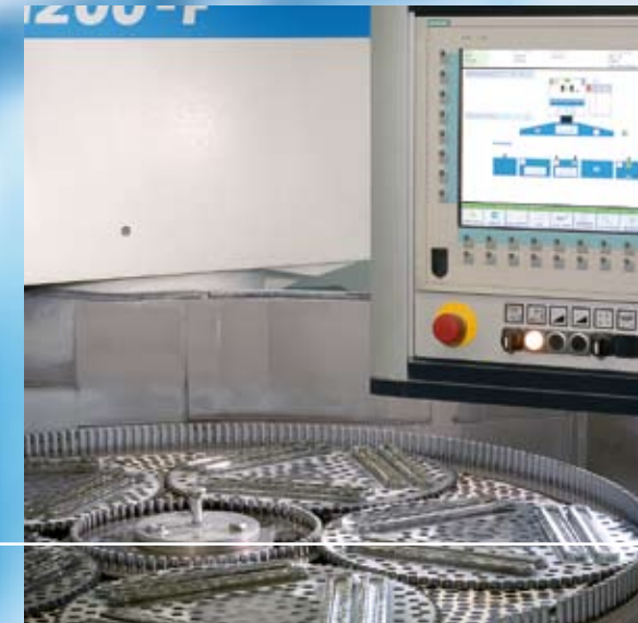
In order to achieve the high final quality we demand, high parallelism and flatness with minimum surface roughness are an absolute "must". To achieve this, the blanks are ground twice between the diamond pellets of our automatic twin-disc grinding and lapping machines before they are carefully polished.
