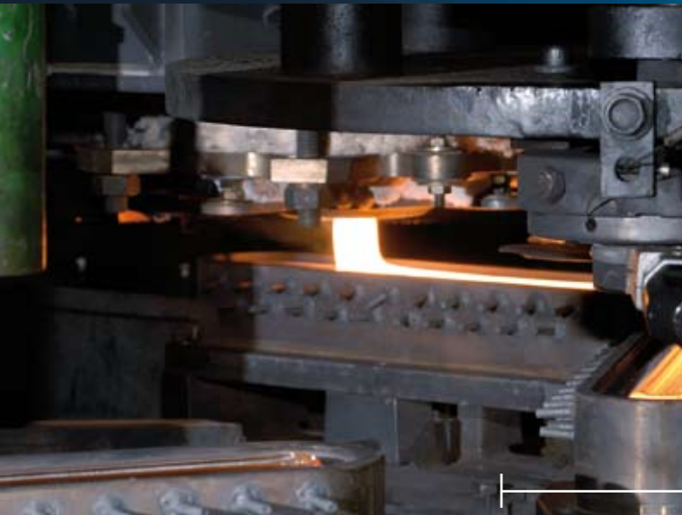
The modern rotary table press gives our sight glasses their shapes.
