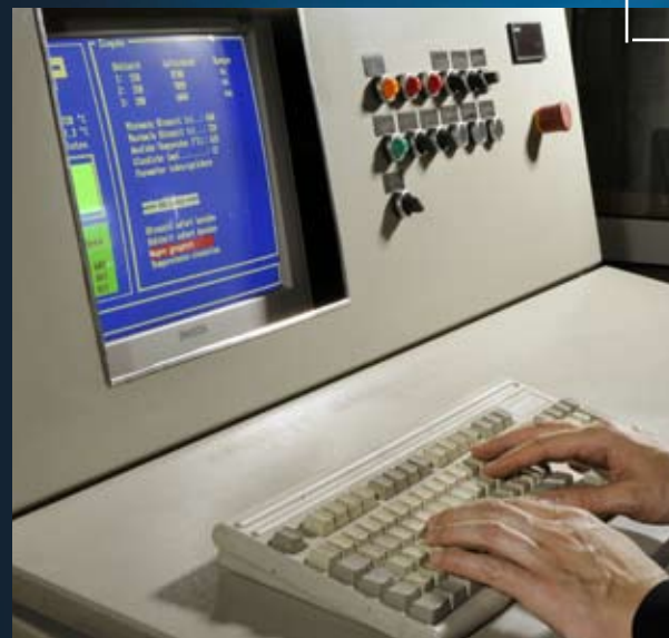
Our sight glasses are subjected to a very special thermal treatment so that they can withstand the stresses they will later be exposed to in use. In the toughening facility, their normal tensile bending strength is increased by a factor of 2 at least. Custom software controls the demanding process of heating and cooling.
